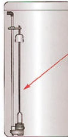
The 464 shut-off prevents air from entering the Combo Unit during the brine cycle. It also protects against brine tank water level overflow.
